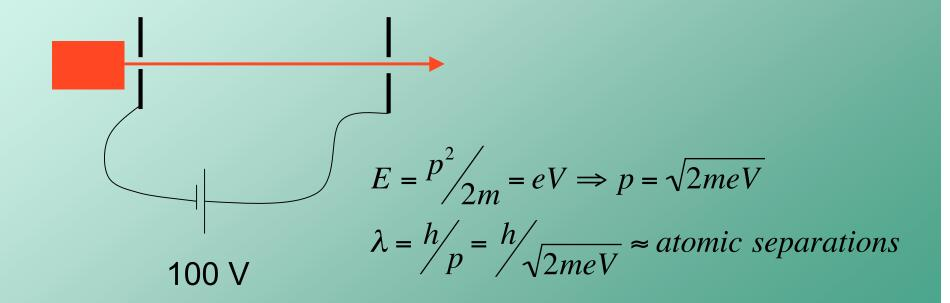
• The elastic mean free path of slow electrons in solids is only a few atomic layers, so elastic electrons remain near the surface.
