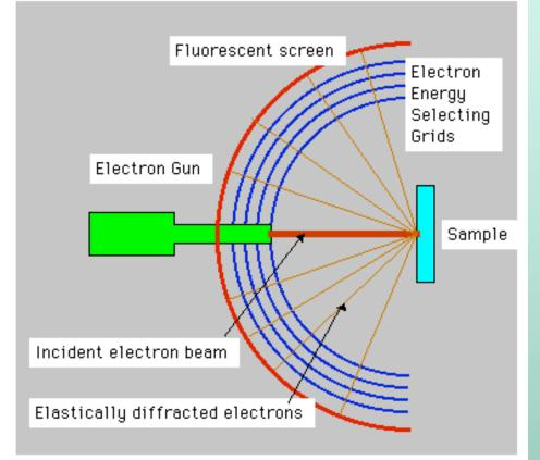
•Low energy electrons impinge on single crystal surface in vacuum
