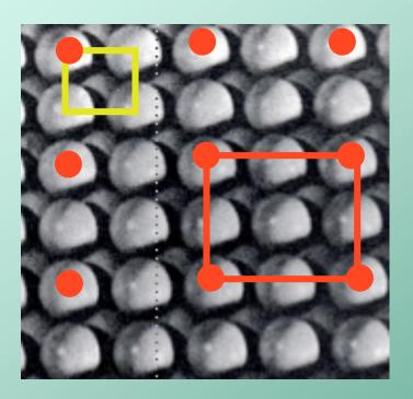
As well as that describing the spatial distribution of the adsorbates if they are present and distributed over the sites in an ordered manner  Spot intensity analysis can be used to determine atoms and their positions within the unit cell e.g. molecular structure of the adsorbate (cf XRD)
